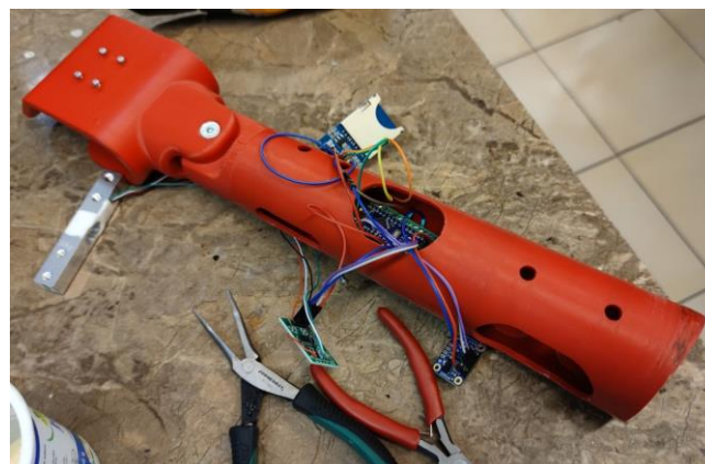
Figure 26. Assembly of electronic components – putting microcontroller in central hole.
