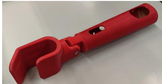
Figure 25. Prosthesis forearm and end effector assembled together.
