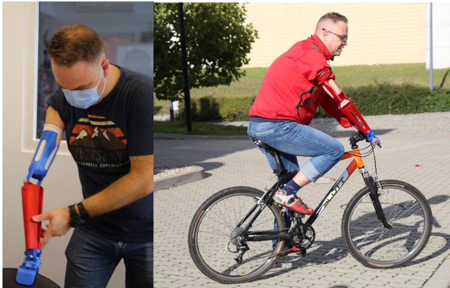
Figure 5. Tests of initial, mechanical version of the prosthesis, a) laboratory tests, b) usability tests
