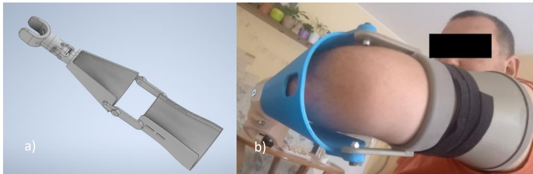
Figure 3.4. Mechanical prosthesis, a) design [15]; b) printed product tested by the patient
