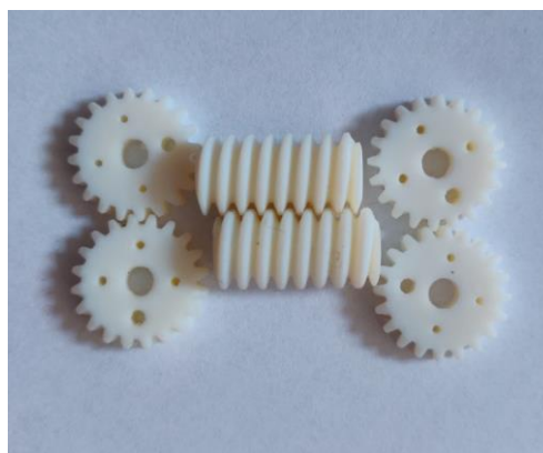
Figure 3.11. Parts printed using PolyJet technology (Stratasys MediJet J5)
