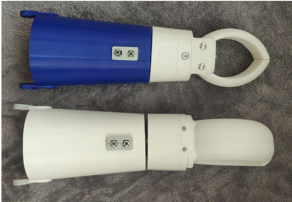
Figure 3.14. Assembled prostheses (without the – arm part), variant 1 (top) and 2 (bottom)
