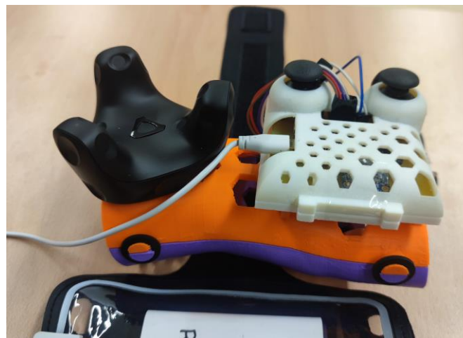
Figure 11. Assembled orthosis with controller, motion tracker, straps and powerbank
