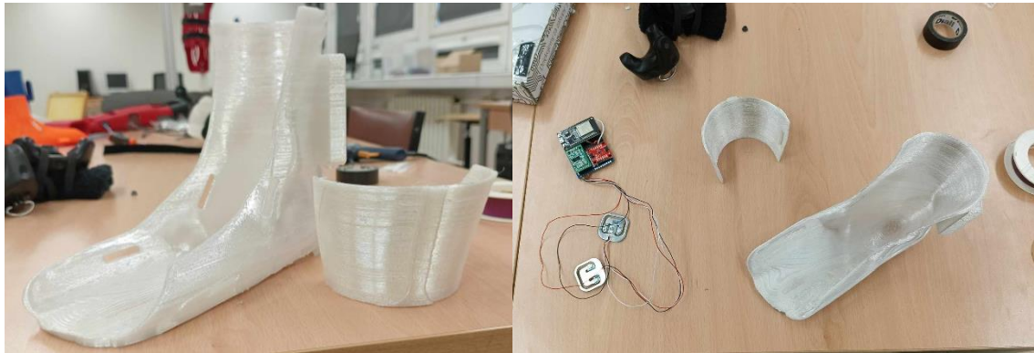
Figure 26. Damaged orthosis as a result of testing left lower limb AFO orthosis
