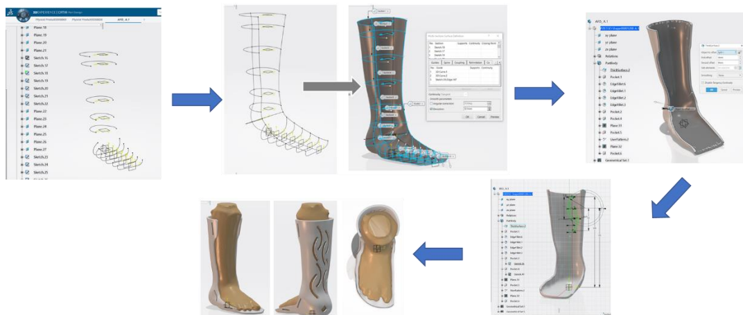
Figure 4. Methodology of creating the lower limb orthosis model based on personalized scans, based on work presented in [2]
