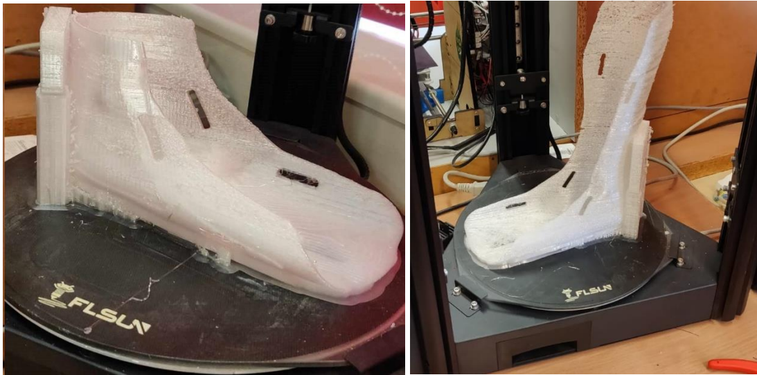
Figure 21. Results of first and second NOK printed orthoses
