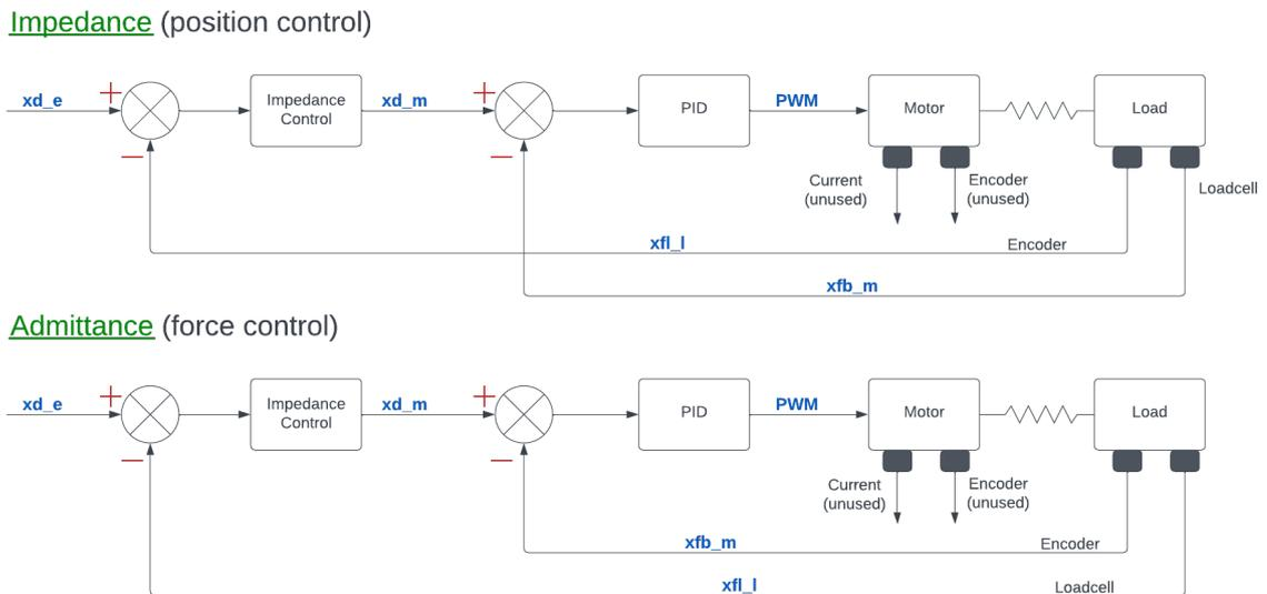
Figure 3.4. Control structure of the robotic haptic arm [1]
