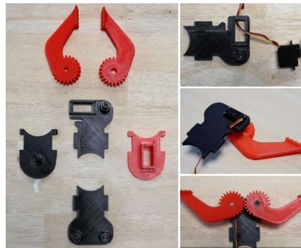
**Figure 2.1.** Robotic arm parts 3D printed using low-cost FDM technology [2]
