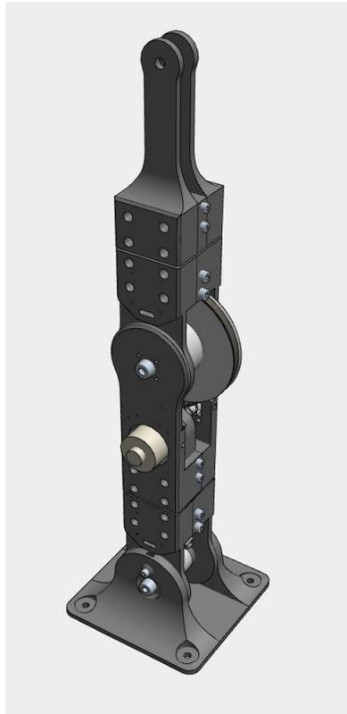
**Figure 3.1.** The robotic gripper 3D design [41]
