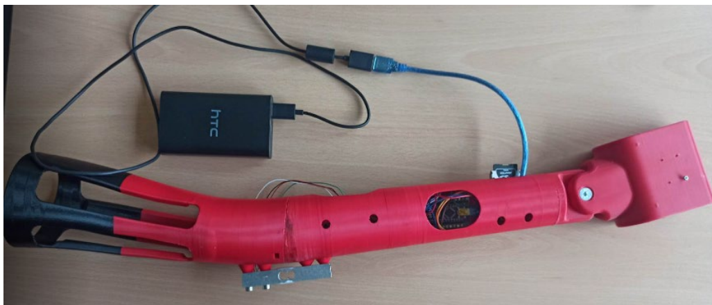
Figure 3.6. Full mechatronic prosthesis [2]
