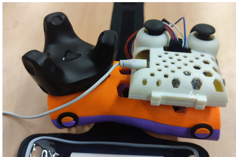
Figure 3.21. Mechatronic orthosis – assembled [6,8]
