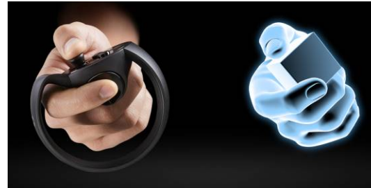
VR controller example, with its virtual representation [oculus.com]
