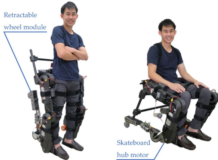
Alpha prototype of a wheel-chair-exoskeleton hybrid robot in standing position (for walking over obstacles) and in wheelchair mode (for safe and energy-efficient movement over smooth surfaces) [28]
