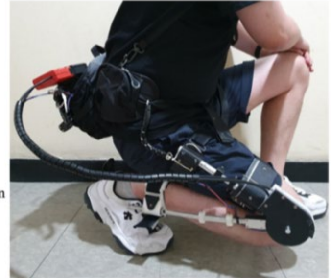
The full appearance of the exoskeleton and the actual wearing appearance, which presents the range of operation. The exoskeleton has three degrees of freedom (DoF). The knee has a flexion/extension DoF, the angle of which is indicated by \theta . In addition, the ankle has a passive rotation DoF and a passive prismatic DoF. The range of motion of the exoskeleton is 145^\circ . The compliant structure allows the user to sit completely [30]
