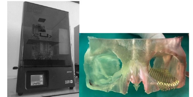
Figure 2.7. Anatomical part printed with SLA (inside the machine) and its clinical use for implant shape adjustment [9]
