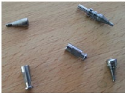
Analogue dental implants manufactured by DMLS
