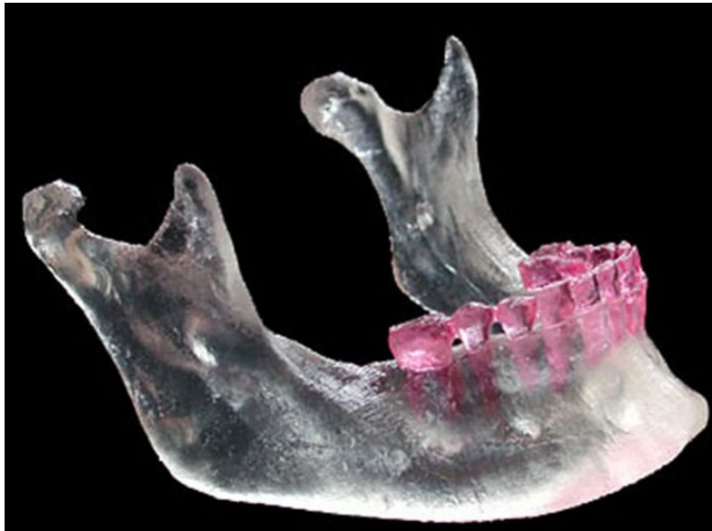
Transparent resins used in dental domain manufactured by SLA
