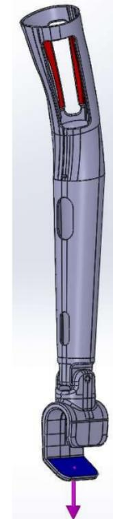
Figure 2: Principle of the distal tensile test simulated for evaluating the strength characteristics of the upper-limb prosthesis (red surfaces – regions where the upper arm is firmly attached to a rigid support; blue surface – support of the traction load)
