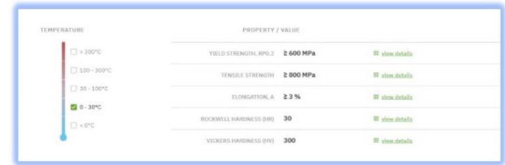
Fig.9. Mechanical properties Ti6Al4V at the temperature between 0-30°C
