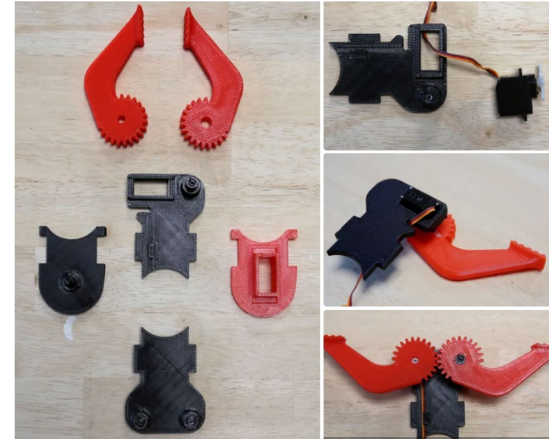
Figure 1. Robotic arm parts 3D printed using low-cost FDM technology
