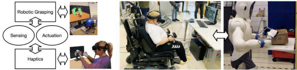
Figure 2.5.25. Sensing/actuation technology and haptic technologies used for teleoperation
