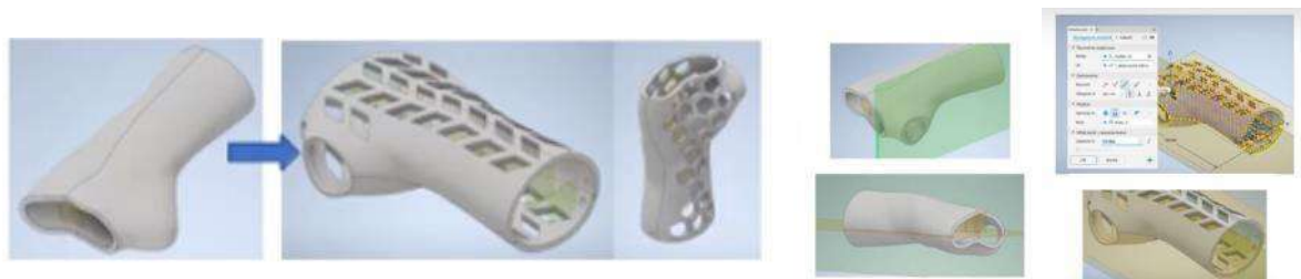
Figure 2.2.32. Cutting operations realized in CAD design to create the part with lattice structure embedded
