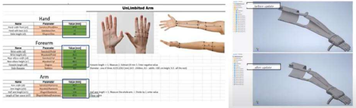
Figure 2.2.31. Parameter settings made using AutoMedPrint system and the updated CAD model with the new settings realized
