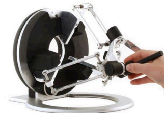
omega.6 pen-shaped force-feedback device
