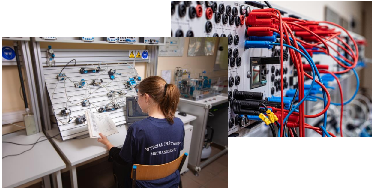
research workstation with hydraulic and pneumatic systems
