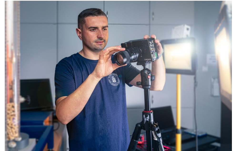
image recording and analysis station equipped with a fast Cronos 1.4 camera and a lighting system
