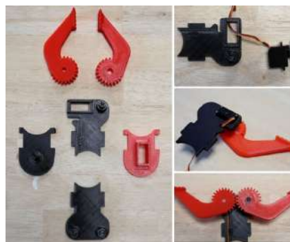
Figure 1. Robotic arm parts 3D printed using low-cost FDM technology [2]
