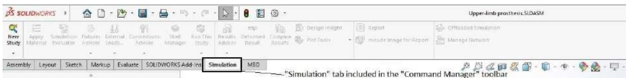
Figure 6: "Simulation" tab included in the "Command Manager" toolbar after the activation of the SolidWorks Simulation module
