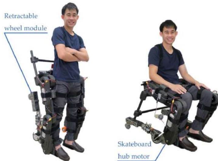
Figure 3.14. Alpha prototype of a wheelchair-exoskeleton hybrid robot in standing position (for walking over obstacles) and in wheelchair mode (for safe and energy-efficient movement over smooth surfaces) [28]
