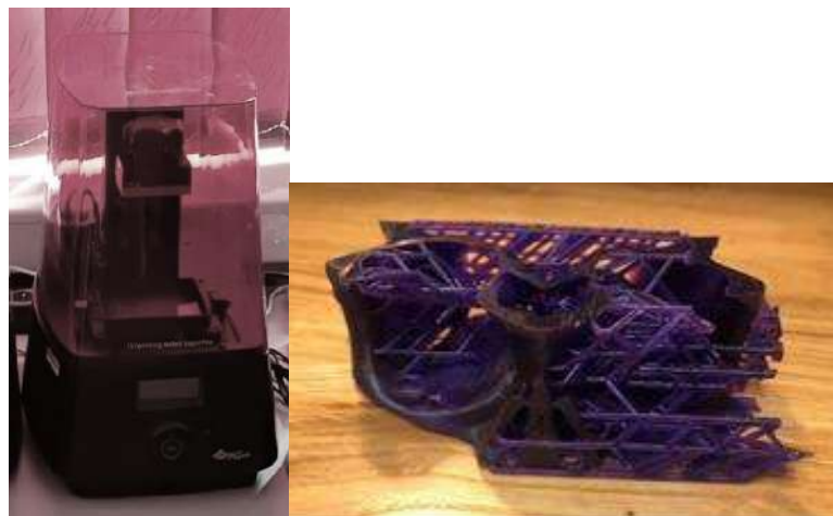
Figure 2.10 DLP machine and example of anatomically shaped product [10]
