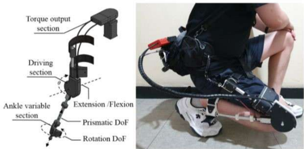
Figure 3.15. The full appearance of the exoskeleton and the actual wearing appearance, which presents the range of operation. The exoskeleton has three degrees of freedom (DoF). The knee has a flexion/extension DoF, the angle of which is indicated by \theta . In addition, the ankle has a passive rotation DoF and a passive prismatic DoF. The range of motion of the exoskeleton is 145^\circ . The compliant structure allows the user to sit completely [30]
