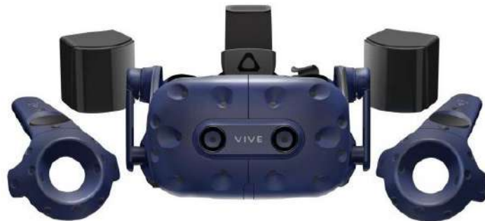
Figure 2.8 Example of a VR headset – HTC Vive Pro – with controllers and base stations [vive.com]
