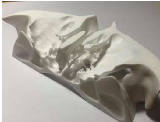
Figure 2.12. Example of anatomical object produced by SLS technique [11]
