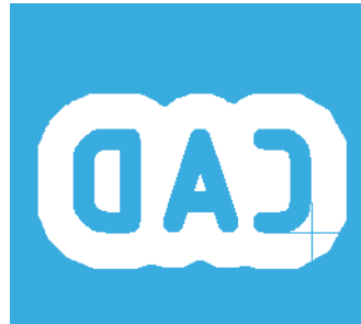
Fig. 3.14 Example of text in bottom copper layer
