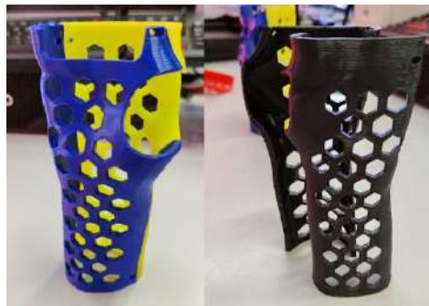
Figure 3.7. 3D printed test orthoses, PLA (left) and TPU (right)
