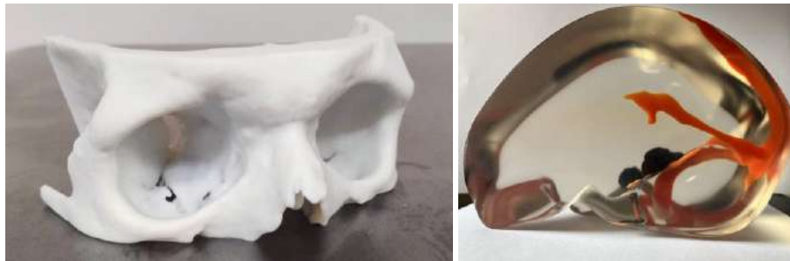
Figure 2.9. Example of anatomical models produced by PolyJet [9]
