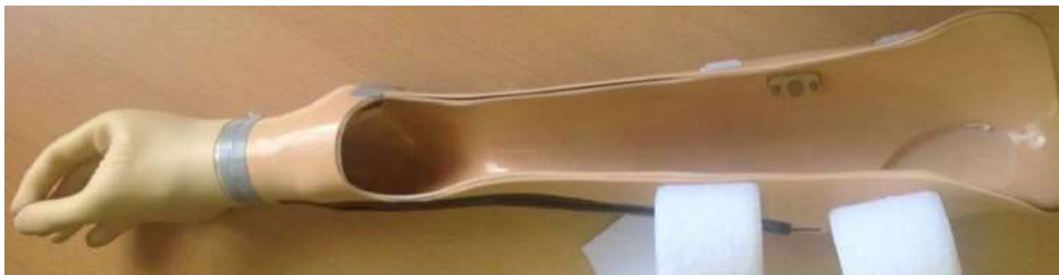
Figure 3.6. A prosthesis simulator for use in anatomically intact individuals. The socket is designed to fit over the forearm and fist. Straps allow the socket to be pressed against the person's arm. It is not possible to customize the electrode placement for each person [22]
