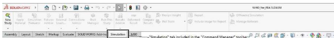
Figure 4.5: “Simulation” tab included in the “Command Manager” toolbar after the activation of the SolidWorks Simulation module
