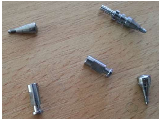
Figure 15. Analogue dental implants manufactured by DMLS
