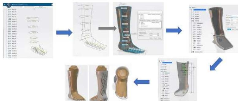
Figure 53. CAD designing step of the orthosis
