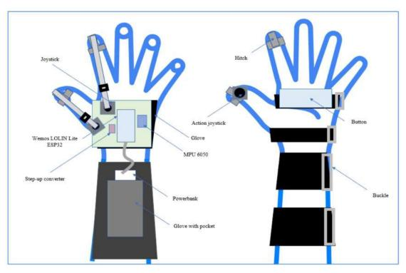
Figure 49. Designing of the controller for the patients with upper limb orthosis
