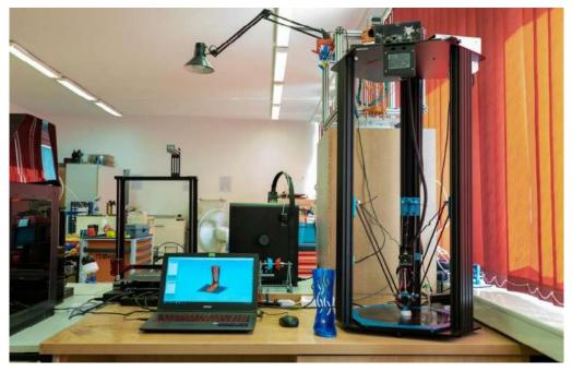
Figure 54. 3D printing process of the realized orthosis
