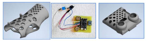
Figure 50. Orthosis and interior / exterior housing part of the controller
