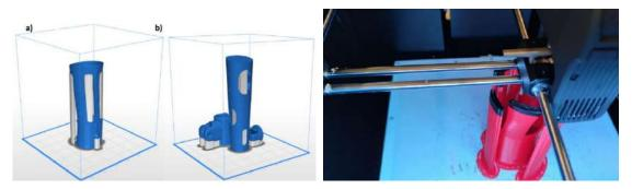
Figure 45. Components of the prosthesis realized by 3D printing
